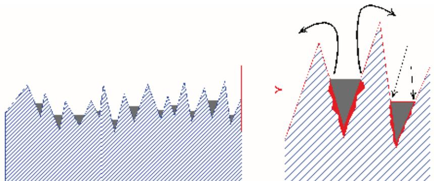
Fig. 9. Ground surface that has been significantly enlarged in the diagram. Dirt and other deposits ensure that chlorine ions, for example, are able to penetrate deeply underneath these depositions leading to local corrosion of the surface. Corrosion products such as rust will then appear.
